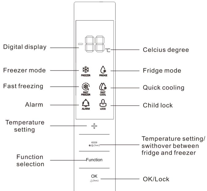
When the refrigerator system is connected to power supply for the first time, all icons on the display panel gets illuminated for 2s, and the system runs in the freezer mode at -18°C by default. When all the doors are close, the display gets extinguished automatically if no key operation within 3 minutes. When the display is off, it will light up if any door is opened or any key is pressed.
