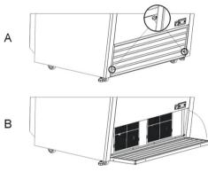
Before beginning with cleaning filter, please make sure the device has been disconnected from power socket. Remove 2 screws from the top of the front grill, see drawing
